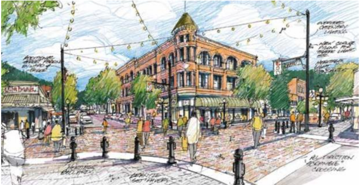
An intersection concept for the central area of Baker Street in Nelson, BC that includes bollards, special paving, overhead lighting, and the potential for an all direction “scramble” intersection with new corner traffic lights.
