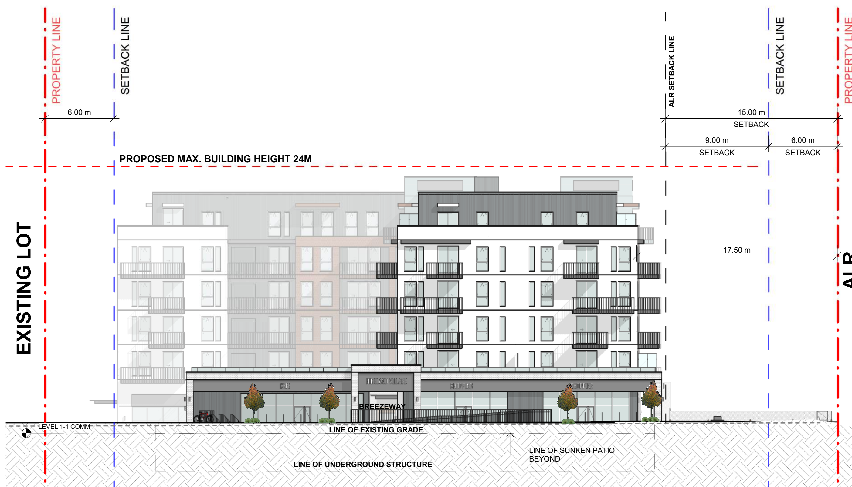
2 SOUTH ELEVATION - RECESSED PATIO OPTION SCALE: 1 : 200
