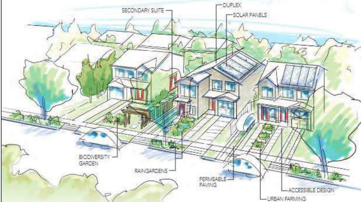
Figure B-6 Artist rendering showing infill and redevelopment on a residential street with climate-friendly design features.
